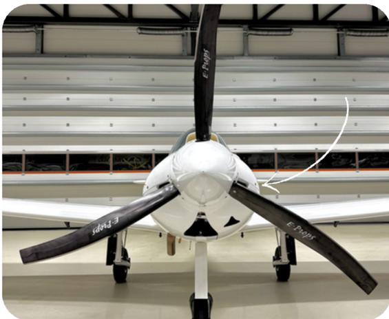
Propeller designed for Rotax 915iS / 916iS engines.
